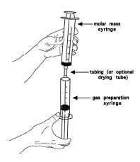
Determine the mass of the MM device plus gas contents. Record the volume of the gas in the syringe by reading the volume from the inside edge of the rubber plunger seal inside the syringe barrel. Record the temperature and barometric pressure.
