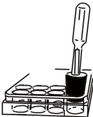
Figure 2. Slater and Rayner-Canham describe the generation of gases in a 24-well plate.
