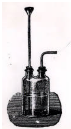
Figure 5. The Wolff's flask was used to prepare a number of gases, including hydrogen [Rensen, 1886].
