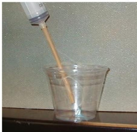
**Variation 1.** Discharge the entire contents of the syringe in a quick manner — within a second. The flame will go out. (The picture shows the gas being discharged in the “incorrect way” according to the discussion in the previous experiment. We usually do not discharge gas in this manner; however in this experiment rapid discharge is crucial.)
