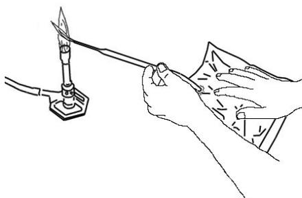
**Option B.** Use of an O<sub>2</sub>-filled gas bag
