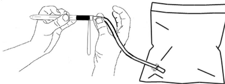
Pour liquid nitrogen into the plastic cup. Hold the bottom third of the pipet in the liquid nitrogen. Within a few seconds the gas bag will start to deflate as the oxygen gas condenses in the pipet. After the oxygen has condensed to a depth of 1 – 2 cm or more, one has a unique opportunity to show the class the pale blue color of liquid oxygen: Do not remove the pipet from the liquid nitrogen as it protects the outside of the pipet from becoming covered with frost.
