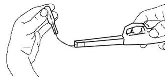
5. Draw some water into the stem — without this, the rocket will not fly far when “launched”. The ends of the wire leads of the piezoelectric lighter must be above the water in the gas-filled region of the rocket. If all of the water escapes, draw a little more up from a cup or beaker of water.
