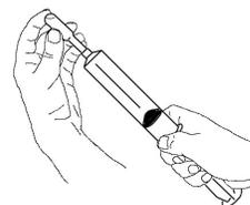
4. Slip the pipet rocket over the wire leads of the piezoelectric sparker. Remember that hydrogen is lighter-than-air! Do not tip the gas-filled rocket open-end up — the gas will escape.
