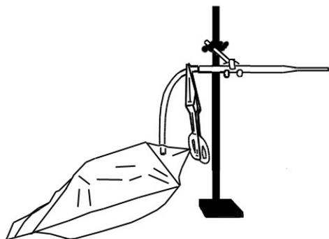
**Figure 5.** The gas bag being used to discharge a flammable gas at a constant rate.
