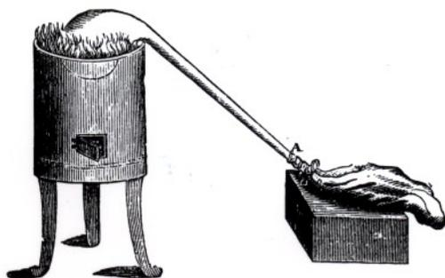
**Figure 2. Gas bladder used by Carl Scheele**
