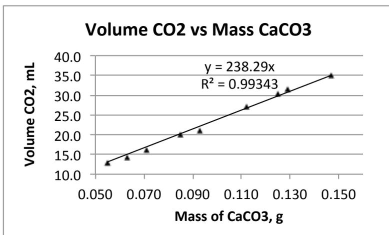
*Volume of carbon dioxide produced as a function of mass of calcium carbonate used.*
