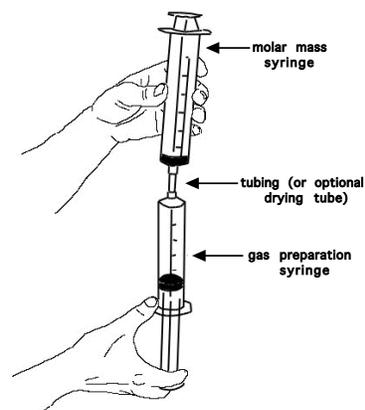
Determine the mass of the MM device plus gas contents. Record the volume of the gas in the syringe by reading the volume from the inside edge of the rubber plunger seal inside the syringe barrel. Record the temperature and barometric pressure.
