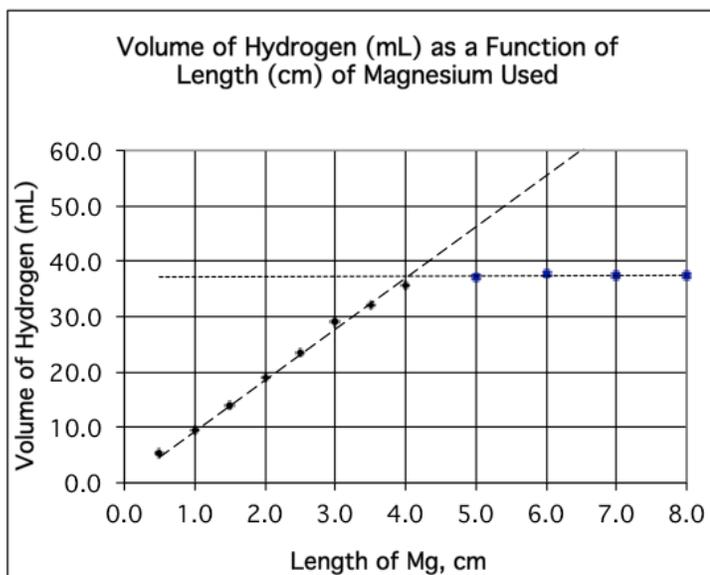
***Volume of H<sub>2</sub> produced as a function amount of magnesium used.***
