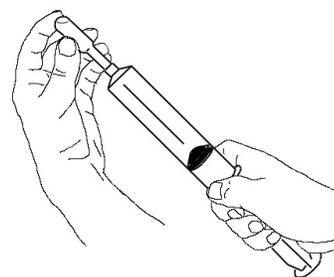
Position the rocket over the wire of the igniter. Water must remain in the stem because this serves as the propellant, but the ends of the wire leads must be above the water in the gas-filled region of the rocket. Trigger the igniter and the rocket will fly 5 m or more. The reaction is:
