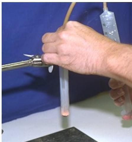
Use the syringe equipped with the tubing/glass pipet attachment to direct the Cl<sub>2</sub>(g) gas in 5 mL increments over the molten sodium from a distance of about 1 cm. A bright, vigorous and short-lived reaction will result. The syringe helps control the direction and delivery of the chlorine gas. The process can be repeated in 5 mL increments of Cl<sub>2</sub>(g) until all of the gas has been used. The reaction is:
