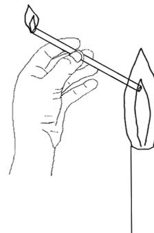
Prepare several syringes full of methane. Two people are required to perform this experiment. One person delivers the methane through the main burner in a continuous, steady stream and ignites the gas issuing from the top. The flame should be large enough that the small tube is positioned towards the top of the flame. Gases diverted into the tube are incompletely combusted and can be ignited by the second person as they issue from the opening.
