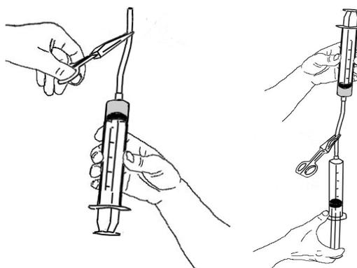
12. Connect the tubing to the silane-preparation syringe as follows. Position the two syringes with the water-filled syringe on top and the silane preparation syringe on the bottom as shown in the figure. Use a ring stand and two clamps (not shown) to
