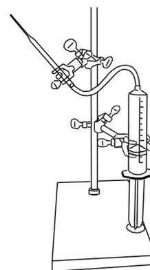
*“silane dispenser” in its proper storage position with the tubing forming a “U” trap airlock*
