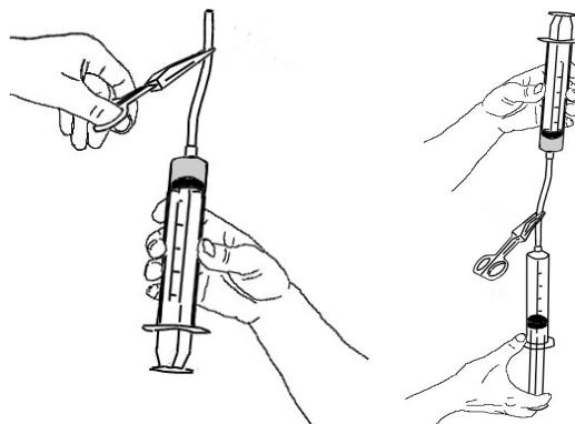
hold the syringes in position. **CAUTION!** Remove the syringe cap from the silane-preparation syringe with a pliers; the contents are likely to be under positive pressure and some flashes of fire with popping noises may be noted. The pliers serves to keep hands a safe distance away. **Caution: Remove the syringe cap with the cap end of the syringe directed upward so that the reagents will not spray out of the syringe.**
