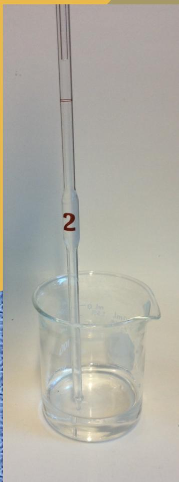
*The last drop in a volumetric pipet is supposed to stay in the pipet. It's been calibrated to work that way.*
