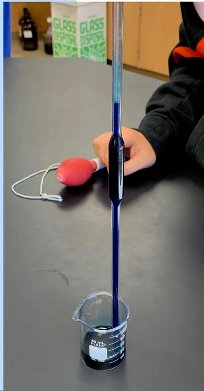
*Start by rinsing the pipet with the stock solution like you see in these two pictures and discarding the rinse solution. You were given plenty.*
