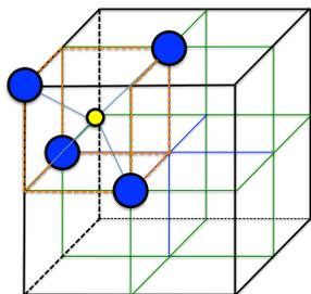
13b. The octahedral holes are along all 12 edge centers and the body-center position for a total of 4.
